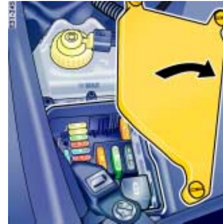
Fuse box in engine compartment
