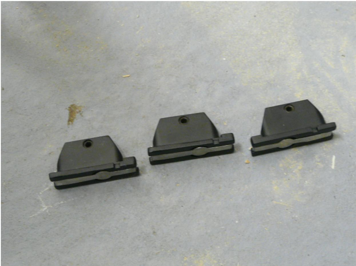
Look below the adapters the adapter marked with "mR" will be the middle adapter, the other two adapters marked "mL" go at each end.
