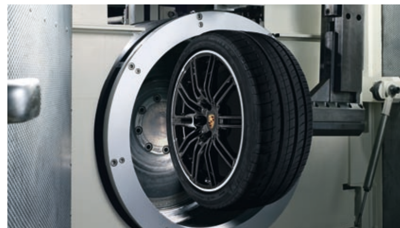
21-inch Cayenne SportEdition wheel painted in black (high-gloss) in the Zwarp test (two-axis test rig)
